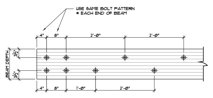
1/2" BOLTS WITH FLAT WASHERS USED THROUGHOUT. DO NOT COUNTERBORE BOLT HEAD/ NUT
